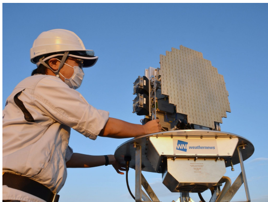
”EAGLE Radar” a compact weather radar for high-frequency observation
